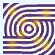
Fail - Wet steam
